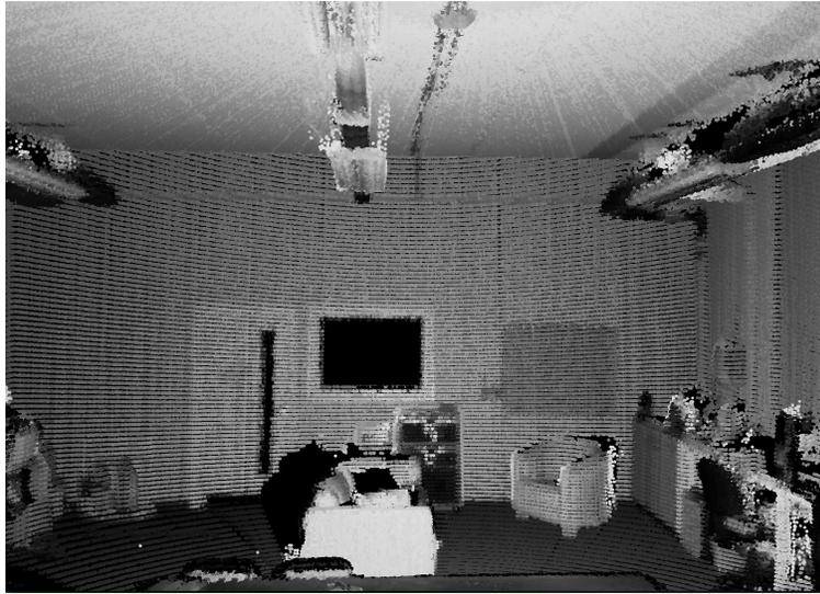
Fig. 8: A crisp point cloud of our lab generated using optimised values  $\hat{\Theta}$ ,  $\hat{\mathbf{H}}$ . Point colouring is based on laser reflectance values. This point cloud was achieved at a laser speed of 1HZ.
